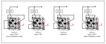
Note: Low Impedance Load examples include incandescent, halogen, resistive loads.
